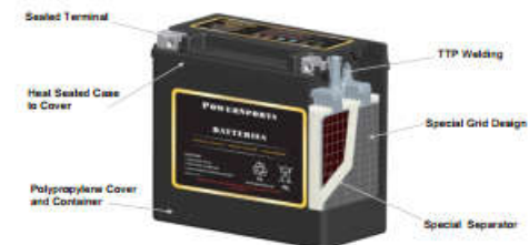
MX Series Factory Activated VRLA (AGM) Maintenance Free Battery (PP)
